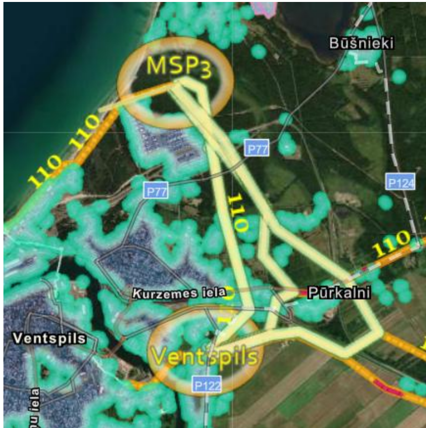
Figure 16. Corridor alternatives compared from Ventspils substation
